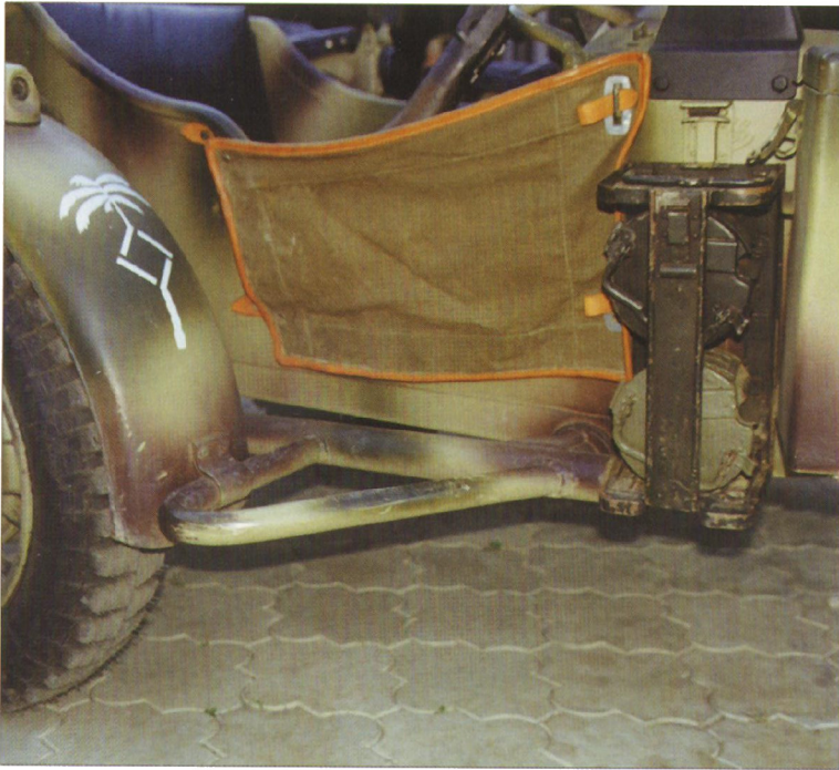
Two basic sidecars were used on Zundapp KS 750 . These were the BW 40 and BW 43 types. Main difference were in springs. BW used wind springs, BW 43 used spring leaves. Seat of a sidecar could be covered by canvas. Behind the seat a voluminous storage space was found.
