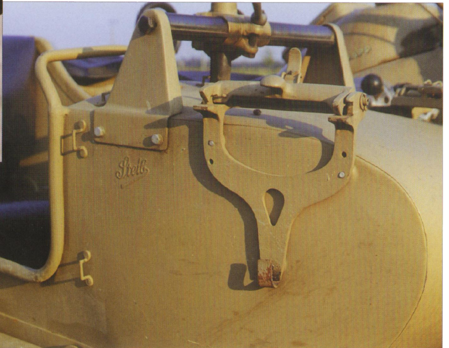
The most famous manufacturer of sidecars was Steib company. All motorcycles were equipped with three map bags on sides of a sidecar. Third was located on left side of a motorcycle behind second seat. First series used leather bags, later metal bags were used.
