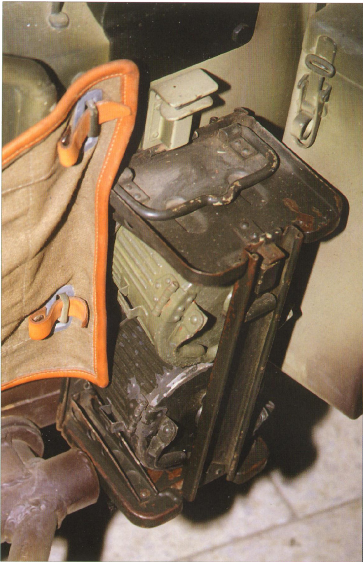
The most famous manufacturer of sidecars was Steib company. All motorcycles were equipped with three map bags on sides of a sidecar. Third was located on left side of a motorcycle behind second seat. First series used leather bags, later metal bags were used.
