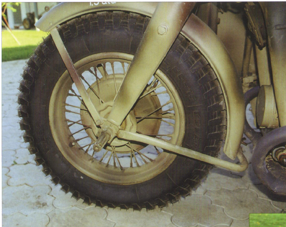
3,00D X 16 front wheel with 4,5 x 16 tyre. The wheel has mechanical drum brakes. 1,5 AtU inscription indicating tyre pressure prescribed.
