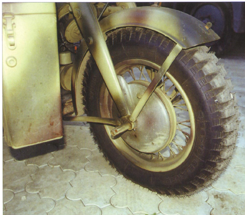
3,00D X 16 front wheel with 4,5 x 16 tyre. The wheel has mechanical drum brakes. 1,5 AtU inscription indicating tyre pressure prescribed.
