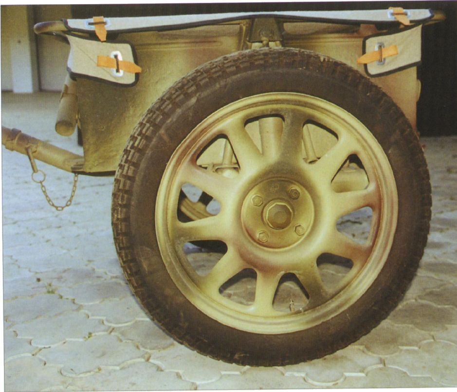
Various manufacturers used different running wheels either with holes or full pressed metal. Trailers were canvas covered.
