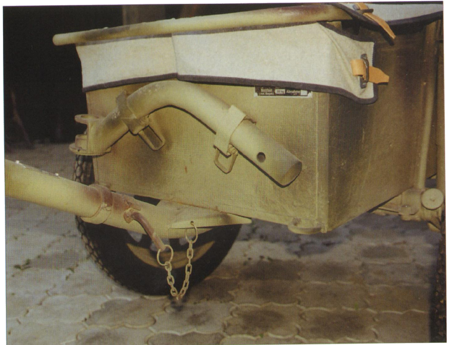
Various manufacturers used different running wheels either with holes or full pressed metal. Trailers were canvas covered.
