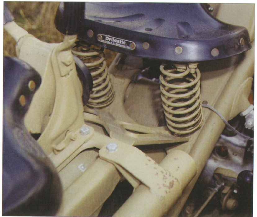
Swinging co-driver's seat was equipped with two upright springs. Co-drivers seat was fixed via two holders and vertical spring - photo below left.
